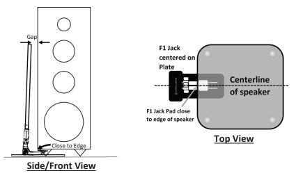
Position the F1 Jack underneath the speaker, centered on top of the floor plate. The speaker may need to be tilted in order to create enough space to slide the F1 Jack underneath it.
